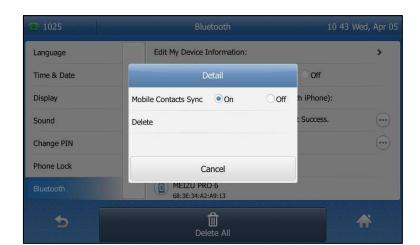
3. Tap the **On** radio box in the **Mobile Contacts Sync** field.
