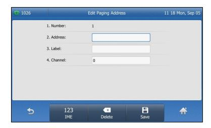
**4.** Enter the multicast IP address and port number (e.g., 224.5.6.20:10008) in the **Address** field.
