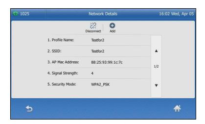
If the IP phone is connected to a wireless network successfully, you can also tap **Wi-Fi Status** to view the connected wireless network information.
