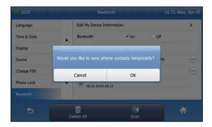
**5.** (Optional.) Tap **OK** to enable the mobile contacts sync feature and the IP phone will sync the mobile contacts temporarily, or tap **Cancel** to disable mobile contacts sync feature and the IP phone will not sync the mobile contacts. If you tap **Cancel**, you can also manually enable the mobile contacts sync feature on the IP phone. For more information, refer to
