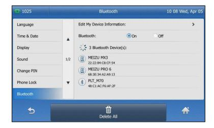
Bluetooth mode is configurable via web user interface at the path **Features->Bluetooth**.
