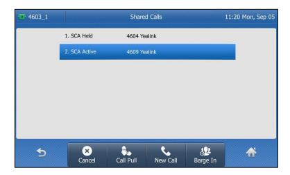
3. Tap the Barge In soft key to interrupt the active call of phone A.
