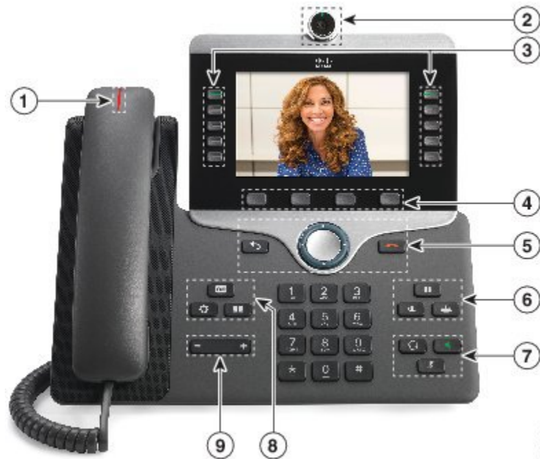
Figure 1: Cisco IP Phone 8845 Buttons and Hardware
