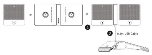
During charging, the battery LED indicator on the CPW90 illuminates solid red. When the battery capacity reaches 100%, the battery LED indicator on the CPW90 will illuminate solid green.
